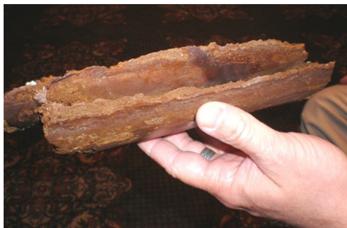
Figure 2. Deposit of iron oxide-infused material extracted from a partially obstructed drainage tile from a golf course in western Pennsylvania. Photo: Peter Landschoot, Penn State
