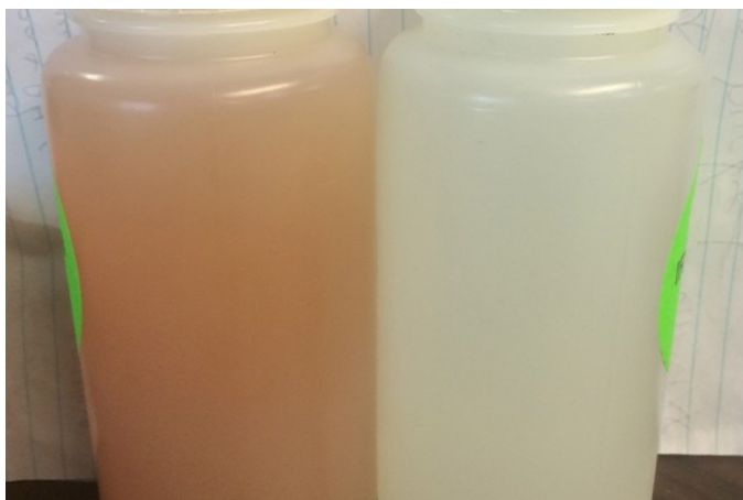
Figure 1. Two irrigation water samples from different golf courses in northern Pennsylvania. The sample on the left (LM-1) shows a reddish-brown or rust color, whereas the sample on right (CO-1) is clear and colorless. Photo: Peter Landschoot, Penn State
