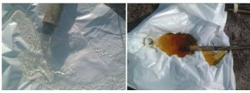
Figure 3. Flush water from treatment of scale using sodium hydrosulfite (left) and citric acid (right).
