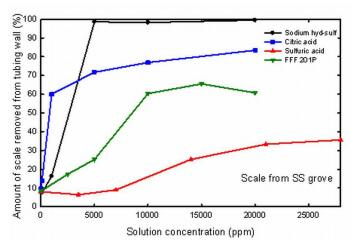
Figure 2. Efficacy of selected chemicals in removing iron scale from irrigation tubing.
