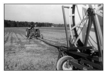
Figure 8. Hose-pull traveler irrigation system.
