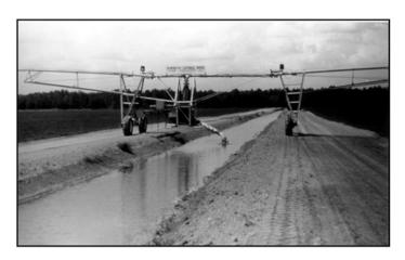
Figure 5. Ditch-fed linear move irrigation system.
