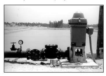
Figure 14. Large agricultural well with electric motor.
