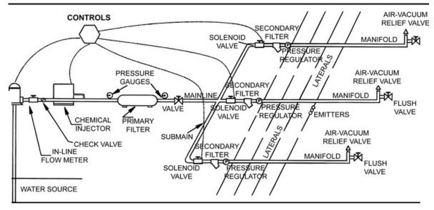
**Figure 10.** Components of typical drip irrigation system.
