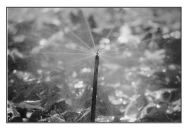
Figure 13. Example of a micro-sprinkler.
