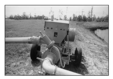
Figure 15. Diesel powered pumping unit on pond.
