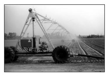
**Figure 6.** Hose-fed linear move irrigation system.
