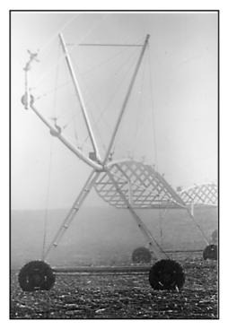
**Figure 4.** Center pivot irrigation system with high pressure impact sprinklers and end gun.
