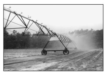
**Figure 3.** Center pivot irrigation system with medium pressure impact sprinklers.
