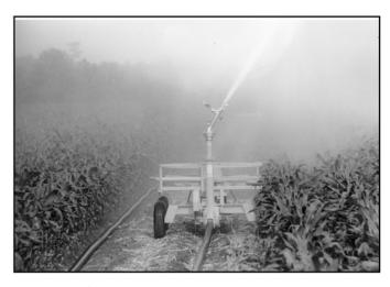
**Figure 7.** Cable-tow traveler irrigation.
