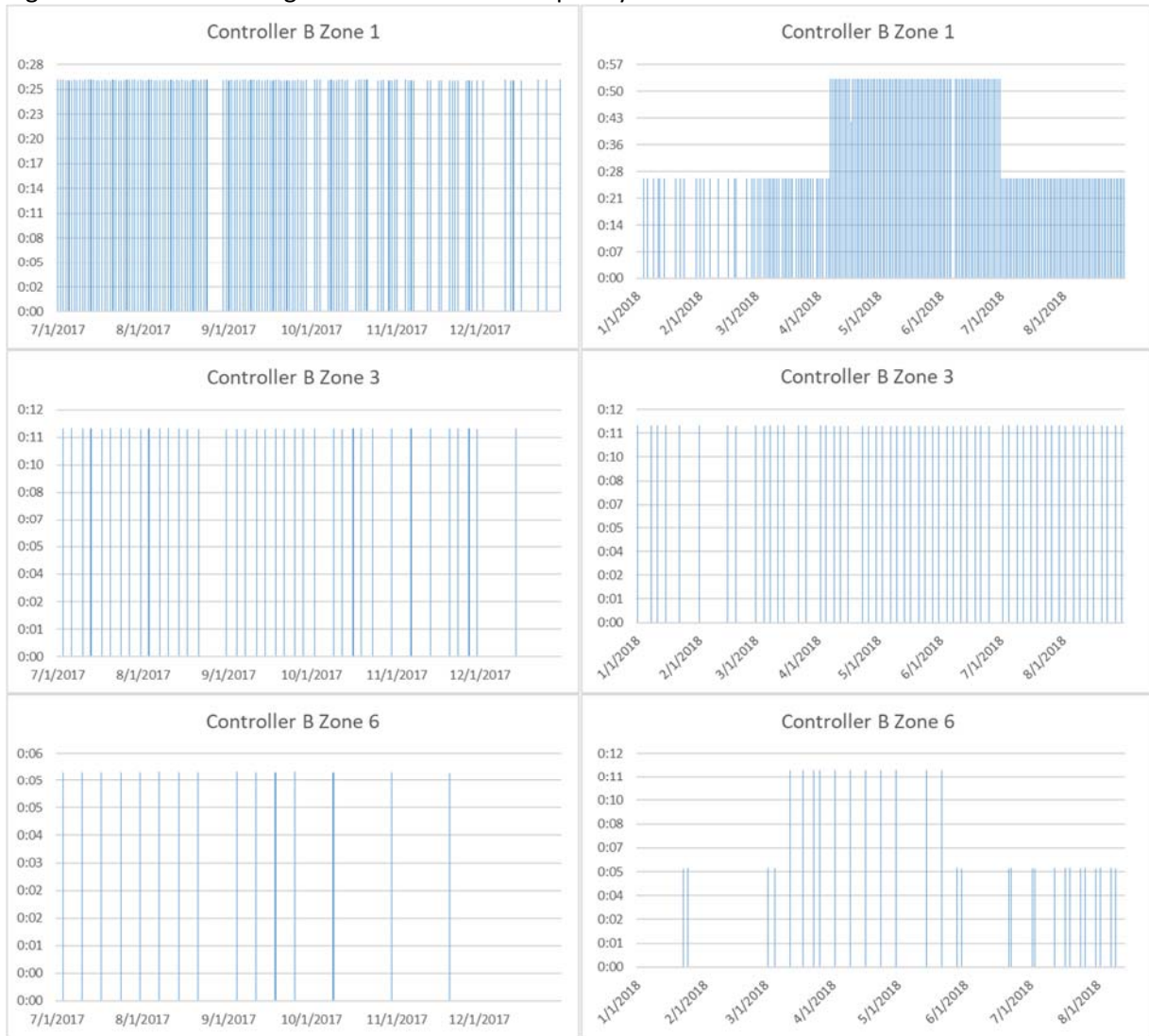
Figure 7. Controller B Irrigation Runtime and Frequency
