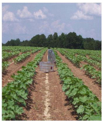
Figure 1. The EASY Pan Irrigation Scheduler in operation on cotton research plots.
