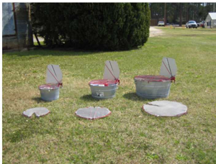
Figure 1. Examples of the three pan sizes used in the test with the 2" wire mesh screen (M~50) on the pans and the window screen in front (M~WS).
