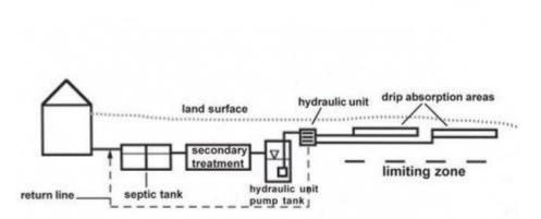
Pennsylvania has approved the use of drip irrigation as an alternate wastewater disposal method for on-lot sewage. The drip irrigation system was developed and is designed for sites with restrictive soil conditions. where the site's limiting zone is within 20 to 26 inches of the soil surface or deeper.
