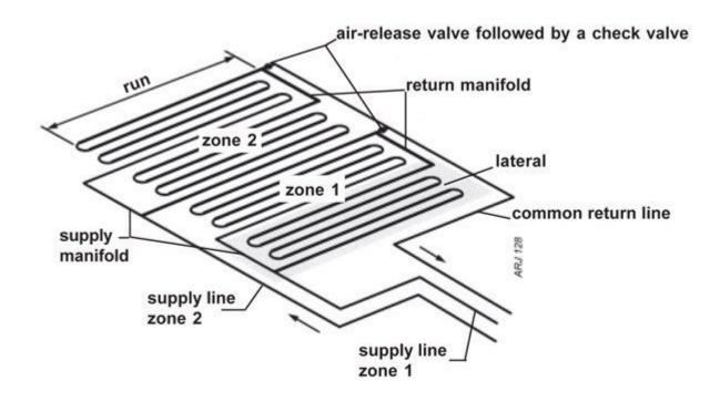
Figure 2. Schematic of drip irrigation zones.
