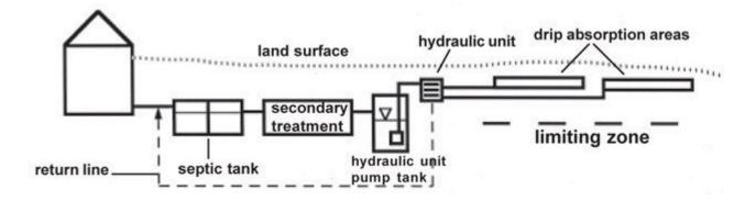
Figure 1. Schematic of a drip irrigation system.
