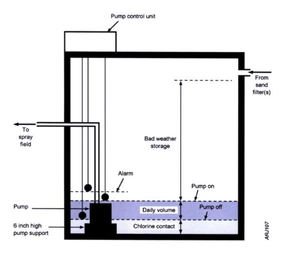
Figure 6. Chlorine contact and storage tank.
