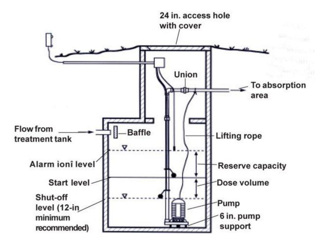
Figure 2. Typical dose tank and pump installation.
