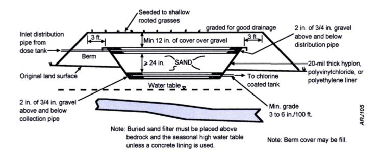
Figure 4. Buried sand filter.
