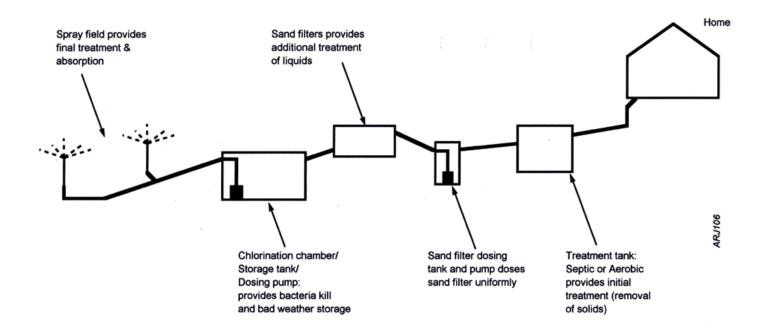
Figure 1. Components of an IRSIS on-lot sewage land application system.
