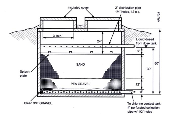
Figure 3. Free access sand filter.
