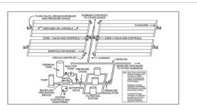
Figure 1. Typical Components of a Subsurface Drip Irrigation System. Mainline, submains, headers, and driplines are below ground. Figure courtesy of Kansas State University.
