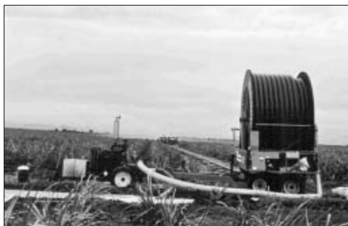
Figure 9. Traveler big gun irrigation system.
