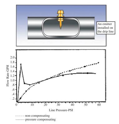
Figure 3. Emitter (above) and performance curve: Pressure compensation for flow rate variation with pressure. The flatter the curve in the 10 to 20 psi pressure range, the better.
