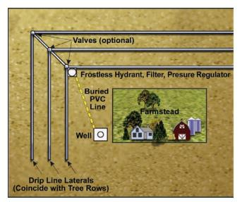
Figure 2. General layout of a windbreak drip irrigation system.
