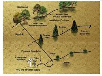
Figure 4. Installation of some components of a typical surface drip irrigation system for windbreaks.
