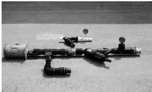
**Screen filters, pressure regulators, and pressure gauges**
