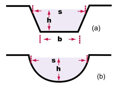
Figure 1. Cross-sectional dimensions for trapezoidal (a) and elliptical (b) ditches. (Diagram by J.S. Jones, 2003)
