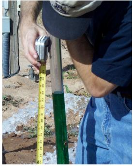
Figure 8. Two photos showing how to measure the head (ft) in a gated pipe system. The head is the distance between the water level in the tube and the center of the pipe. These are Rite-Flow<sup>™</sup> gates and there is about 3 ft of head. According to Table 8, the flow is approximately 39 gpm per gate.
