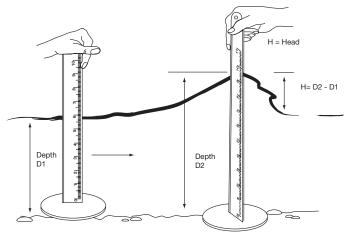
Figure 2. Using a velocity Rod. (Waterwatch, 2002).
