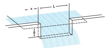
Figure 4. Diagram of a rectangular weir where L = width of weir opening (4 to 8 times H), H = head of weir (measured 6 ft upstream of weir) and  $a = at least 3^{*}H$ .
