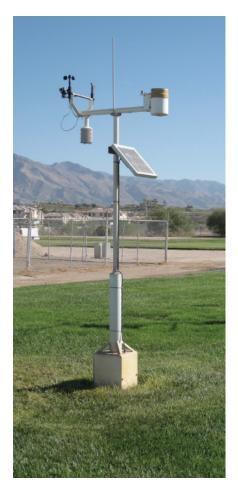
Figure 1. An automated weather station commonly used to estimate turf ET.
