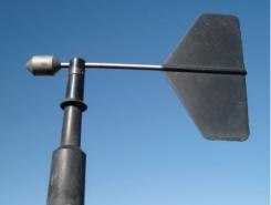
Figure 4. Wind speed is usually measured with a cup anemometer (above) while a wind vane (below) is used to monitor wind direction.
