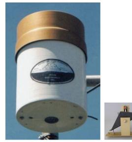
Figure 5. A tipping bucket rain gauge used to measure precipitation. The bucket mechanism (right) tips when a known volume of precipitation falls, triggering a switch closure which is recorded by the data logger.
