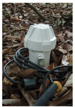
Figure 5. Multi-sensor capacitance probe installed in a south Florida grove.
