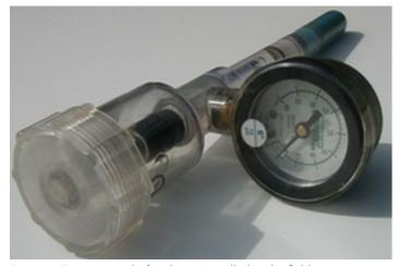
Figure 2. Tensiometer before being installed in the field.
