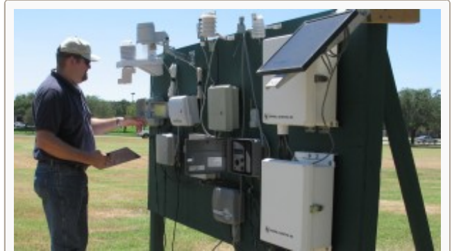
Charles Swanson checks the setup of smart irrigation controllers at a College Station test site. (Texas AgriLife Extension Service photo by Jose Lopez)
