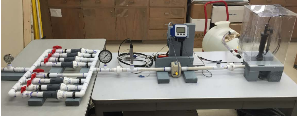
Indoor Pressure/Flow Sprinkler Testing Set Up
