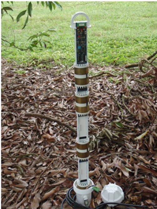
Figure 4. Multi-sensor capacitance probe being inserted into field.
