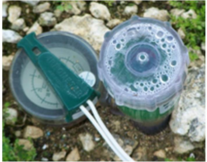
Figure 3. Tensiometer installed in very gravelly loam soil.
