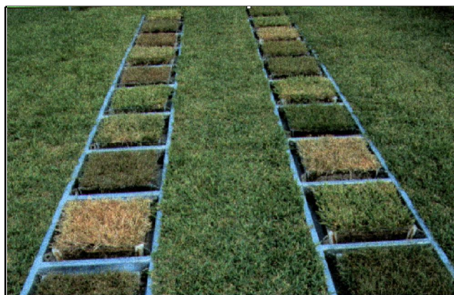
Figure 1. Turfgrass grown at different reduced irrigation rates. Turfgrass is grown in closed containers with an automated rain shelter so only irrigation water is used by the plant.
