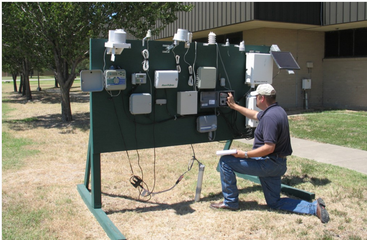
Charles Swanson, Texas A&M AgriLife Extension Service irrigation specialist, checks the setups of the many smart irrigation controllers at a College Station test site. (Texas A&M AgriLife Extension Service photo)
