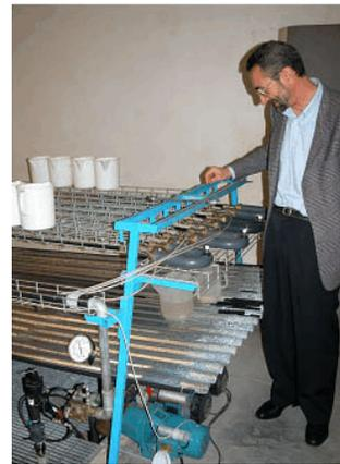
Bertolacci shows bench test apparatus for drip tubing
