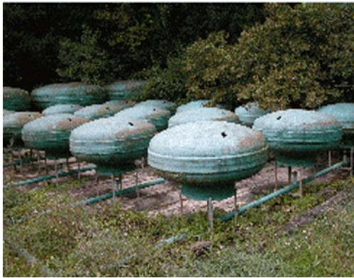
Bank of sprinkler testing containers at the CEMEGREF Lab in France
