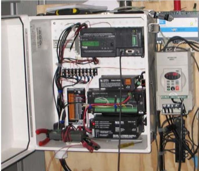
Figure 8. The control system consists of a datalogger and a PLC.
